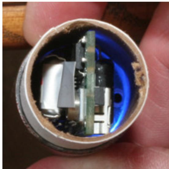
Important: Align the two bulkheads so that they are facing the same direction. If the labels are not facing the same direction, the charges will be connected to the wrong terminals. Attach the shock cord and deployment charges as you did for the other end of the av-bay. Completed av-bay shown below.
